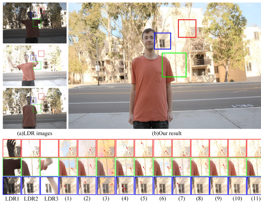
Fig. 1. Performance comparison of the reconstruction results of three LDR images involving the wide-range movement of the targets obtained by different methods. (a) three LDR images are to be fused with unaligned image contents. (b) the reconstruction result obtained by the proposed method. The images shown in the three rows below (a) and (b) compare three local areas extracted from three LDR images and the reconstruction results obtained by different methods. Three enlarged local areas (marked in red, blue, and green frames) extracted from LDR1, LDR2, LDR3, the reconstructed images obtained by (1) Sen [10], (2) HDRCNN [1], (3) SingleHDR [6], (4) Kalantari [11], (5) DeepHDR [12], (6) AHDRNet [13], (7) NHDRNet [14], (8) HDRGAN [15], (9) HDRI [16] and (10) the proposed SGARN, and (11) the ground truth are shown from left to right.
