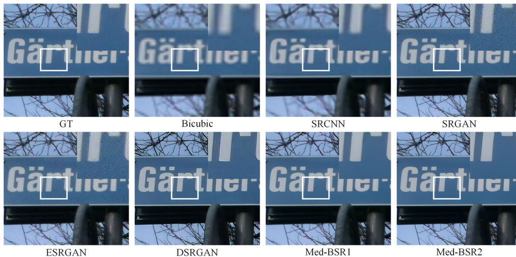
FIGURE 11 Comparison of x4 reconstruction results of natural images by different SR methods
