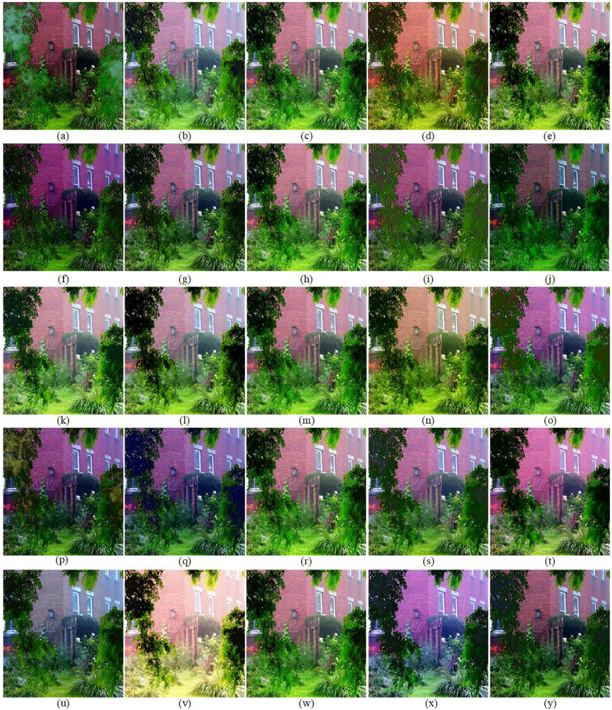
Fig. 13. Effect of hyper-parameters on the dehazing quality of the real hazy image. (a)–(e) \alpha_1 = 0.75, 1, 1.25, 1.5, 1.75 , (f)–(j) \alpha_2 = 0.001, 0.01, 0.1, 1, 10 , (k)–(o) \beta_1 = 0.75, 1, 1.25, 1.5, 1.75 , (p)–(t) \beta_2 = 0.001, 0.01, 0.1, 1, 10 , (u)–(y) \gamma = 0.1, 1, 10, 100, 1000 .
