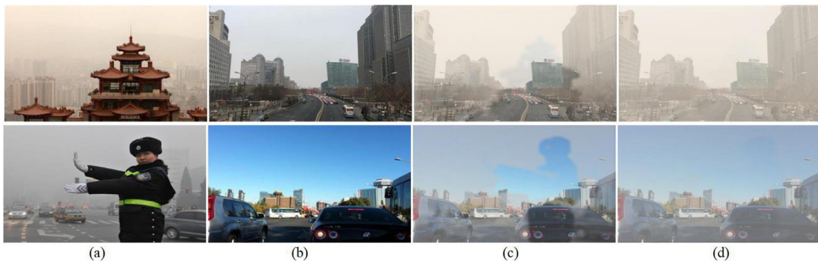
Fig. 10. Generated hazy images by the proposed method: (a) real hazy image, (b) clear image, (c) generated hazy images by the proposed method without discriminators, (d) generated hazy images by the proposed method with discriminators.
