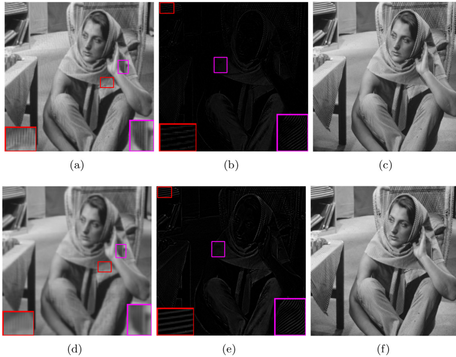
Fig. 3. The effects of our learned dictionaries and image decomposition algorithm. (a) and (b) Low-rank and sparse components of “barbara” image generated only by the learned dictionaries; (c) the result of reconstruction by adding (a) and (b) (with PSNR = 68.8462); (d) and (e) low-rank and sparse components of “barbara” image generated by Algorithm 2; (f) the result of reconstruction by adding (d) and (e) (with PSNR = 74.0158).
