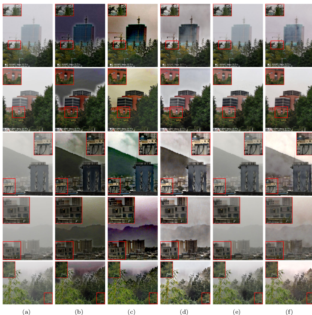
Fig. 4 Comparison of experimental results with different methods. a Hazy image, b DCP, c NLD, d DA-Net, e FFA, f proposed method
